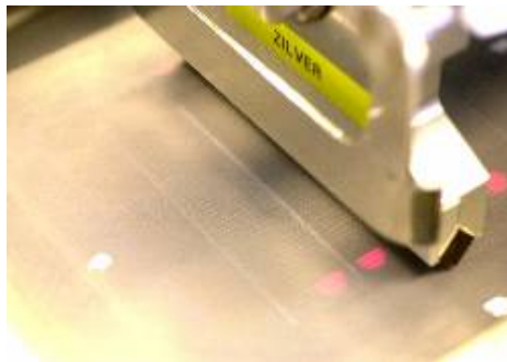
screen printed metallisation
