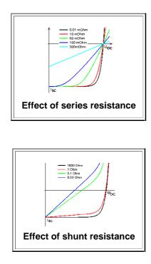
Switching solar cells with individual characteristics in series and / or in parallel causes all kinds of problems.
