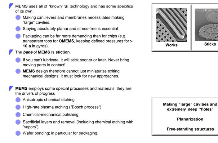
Process integration looks simple if compared to an advanced CMOS process, but is actually rather involved due to the special processes needed and quality requirements
