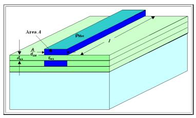
Let's look at a typical AI or Cu conductor on a chip with a length of 1 cm, a cross-sectional area of 0.5  $\mu$ m<sup>2</sup> and the specific resistivity of <u>a typical metal of about</u> 2  $\mu$ Ωcm. The total resistance of our "wire" then is
