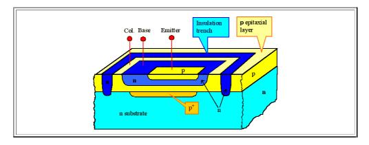
We start with an **n**-doped wafer (of course you can start with a **p**-doped wafer, too; than everything is reversed) and diffuse the **p**<sup>+</sup> layer into it. We will see what this is good for right away.
