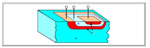
This would be fine in terms of insulation, because now there is always a **pn**-junction between two terminals of different transistors which is always blocked in one direction for all possible polarities.
