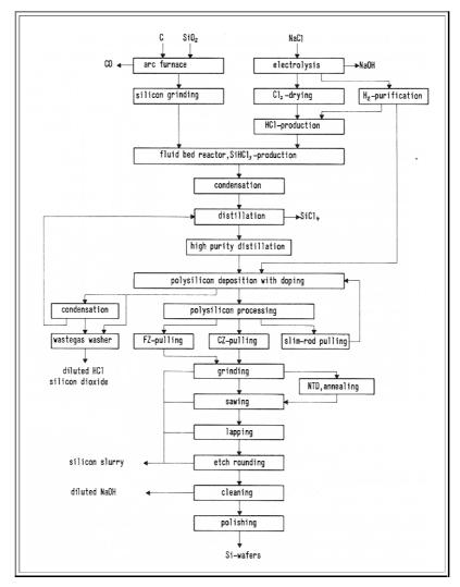
Next, we have a pictorial representation of just crystal growth and wafer production. Again, it contains some self-explanatory processes not introduced before.
