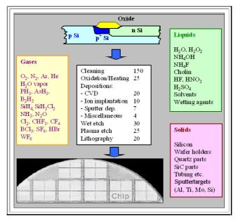
We don't have a chip yet - we only have unpackaged chips on a wafer.
