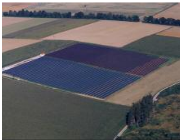
Figure 1: PV Plant “Waltenhofen” with a 400kWp PV subfield with MHI modules (TF; upper half) realized by Phönix and a 720kWp PV subfield with BP modules (c-Si) realized by BP Solar in 2003/2004.
