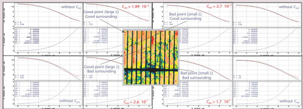
Fig. 6: Fitting of local IV-curves using CELLO  $dI(U_n)$  - data
