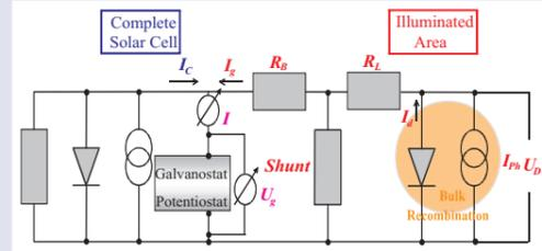
Fig. 2: Equivalent circuit for CELLO measurements
