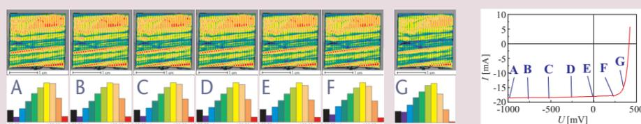
Fig. 7: Lock-in Currents and its relative changes along the IV-curve
