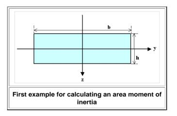
Now apply a force in the z-direction, It bends this rod downwards in the z-direction. For this case I then need the area momentum ly of the rod. The index is "y" because the vector going with the torque or momentum for bending lies in in the y-axis. Bending in y- direction needs lz. The two area momentums ly and lz are defined by:
