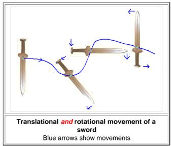
We have the simple picture from above but now the sword translates *and* rotates. You would have to apply proper (and somewhat crazy) forces that also produce torques to cause such a movement, and calculating what it would take to cause such a movement is actually not all that easy.
