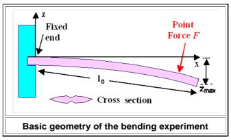
We know that for a given force acting on the blades as shown above once more, the amount of bending or maximum deflection (given by the distance zmax) increases
