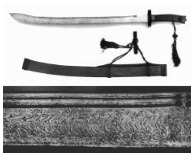
Figure 8. A 17 th century Chinese sword of the pattern-welded variety. The pattern shown on the macrograph arises from the difference in etching of the two dissimilar steels from which the sword was manufactured, involving a solid-state bonding process. Courtesy of the Metropolitan Museum of Art, New York. [17]
