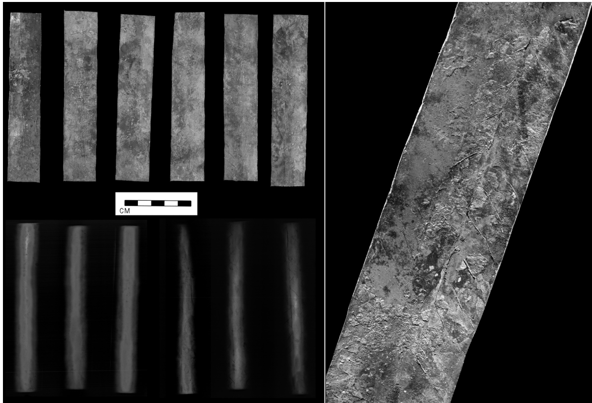
Fig 2. Photograph (top) and corresponding X-radiograph (bottom) of the six blanks used in this study: first three blanks are from sample NPW and the last three blanks are from sample PW. The design of PW can be seen in the accompanying close-up image of the surface of one of the blanks (right).
