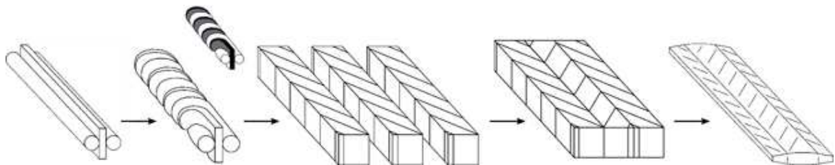
Fig 1. A diagram showing the stage by stage process for the pattern-welded construction of PW. The flat strip that is twisted with two rods (used to make a bundle) is highlighted in grey in the smaller image accompanying the second stage. Three bundles are finally welded and forged together.
