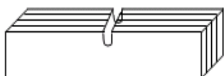
Fig. 3. Test specimen for U-notch Charpy impact test. The notch direction is perpendicular to the layers running
