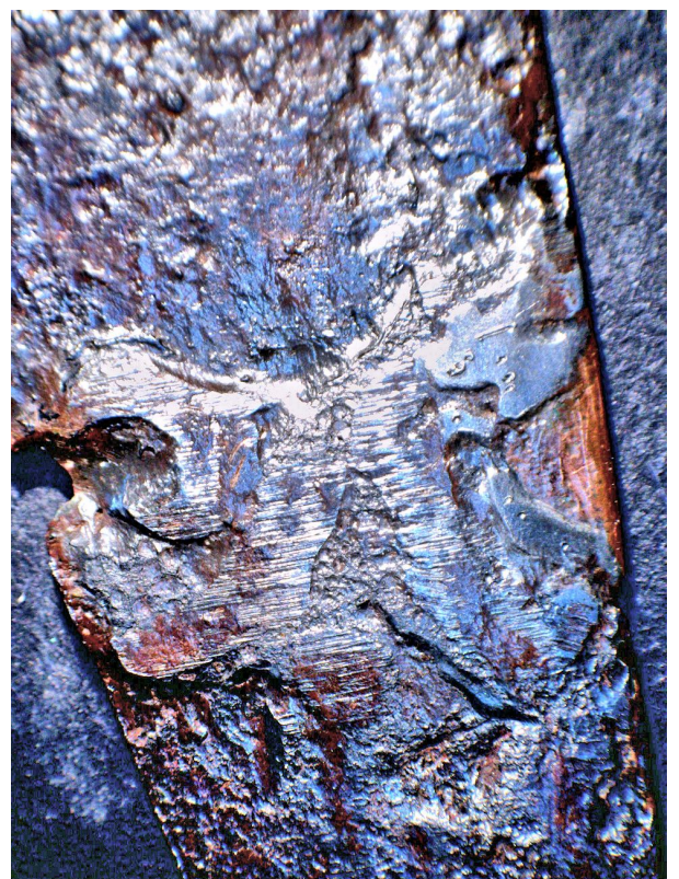
Peculiar "s,eared" strucre across the blade at the position of the small inset.
