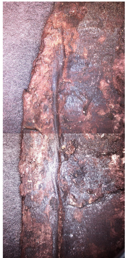
Wormhole (around position 17). Its diameter is about 0.8 mm.
