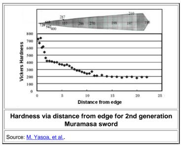
It is not clear, however, if hardening with a clay coating has been used; no mention of the hamon is made. It is also not clear if piling was used and what kind. The pictures given do not show faggoting. The authors refer to faggoting though, but in a nonsensical manner ("The grain size of sharp edge part is observed to be very fine, about 10-15 µm as a result of the effect of 10 several times-forgings in sword making process").
