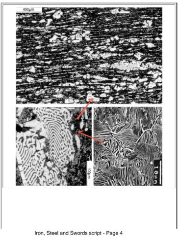
Top: Broken up and banded cementite in a plate of tamahagane fire welded from a number of smaller pieces. Bottom: The fine structure of the cementite particles and the pearlite in between. Note change of scale
