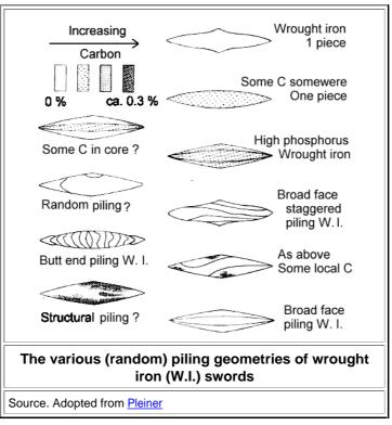
Note that one or two cross-sections are not necessarily representative for the whole length of a blade. But what becomes clear in any case is that Celtic smiths used many different ways to construct sword blades by fire or hammer welding wrought iron or mild steel bars. Some piling might have been random, in other cases the smith might have made an attempt at structural piling but essentially failed.
