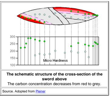
The black lines mark weld seams (not always clearly discernible), the colors the rough carbon concentration. In addition, micro-hardness values are given for the positions indicated.
