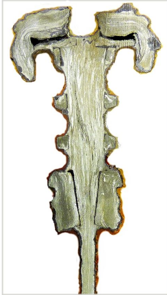
Luristan iron mask sword cut in half and etched for structure revelation
