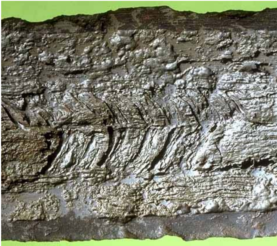
5. Detail of a winged spearhead, 9th century Carolingian type, showing remains of two thin bands of pattern welding of diagonal form, forming a chevron, overlying a base of non-patterned metal. Wide bands with relatively straight pattern are frequently thin, suggesting much flattening of the rods ( Private collection ).
