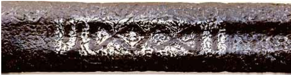
9. Detail of an +ULFBERHT+ inscription and geometric designs on the opposite face of the blade, 10th century. Notice the patterns within the twisted rods used to form the inlay. (Private collection).
