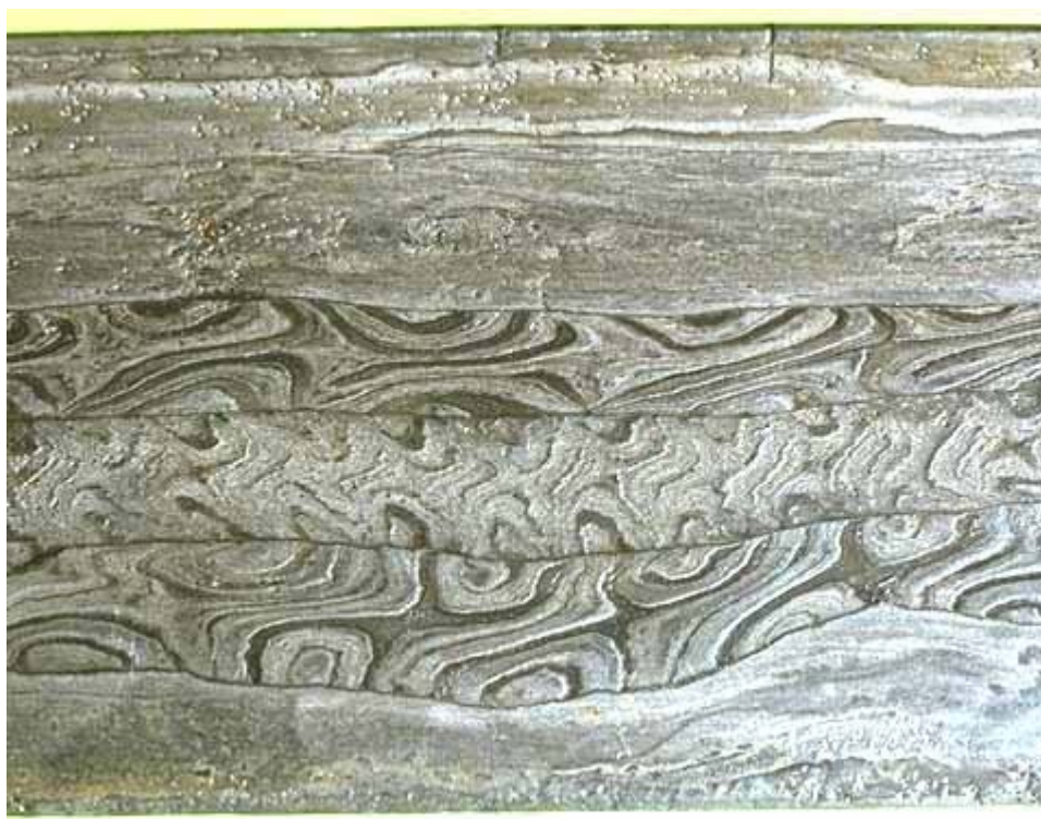
4. Detail of a yataghan blade, probably 18th or 19th century, showing three bands of pattern welding, exposed to varying depths generally between 25 and 50% of the rod thickness. The blade is relatively thin except for a ridged back and differences in the courses of the bands hint that there are three separate strips applied to each side and that the pattern-welded rods may have been flattened considerably ( Private collection ).
