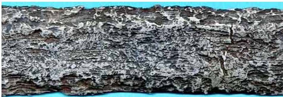
7. Detail of a double edged sword, 8th to 9th century. The central portion of the blade is composed of four bands of pattern-welding and shows straight areas alternating with pattern consistent with being from the center of the rod. As areas of corrosion not pictured disclose a central plain core, the blade contains a total of eight patterned strips. To the right of the center, perpendicular to the long axis a stress crack is seen crossing the bands; the other layers of the blade appear to have better withstood the stress ( Private collection ).
