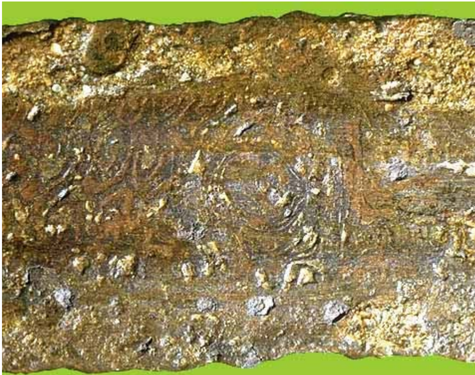
8a. Detail of a double edged sword blade found in the Netherlands showing background curved patterns on the left, consistent with a plane of section nearing the centers of the composing rods, and having a central circular overlay in iron, to the right of which is another overlay perpendicular to and overlying the fuller; probably 8th or 9th century. (Private collection).
