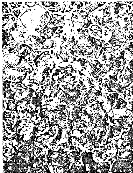
2.41 Transition between high and medium carbon area in handle, immediately below pommel of No. 104 (Cf. Figure 2.16C). Etched, 96X.
