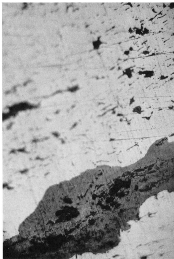
FIG. 6. Polished section of tip of beard, before etching, x 200
