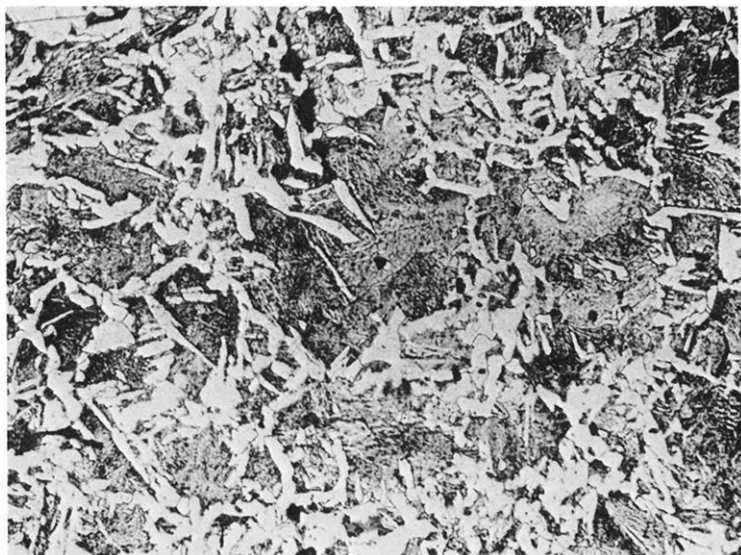
FIG. 5. Polished section of pommel disc x 200. Ferrite and pearlite in steel about 0.5% carbon. British Museum
