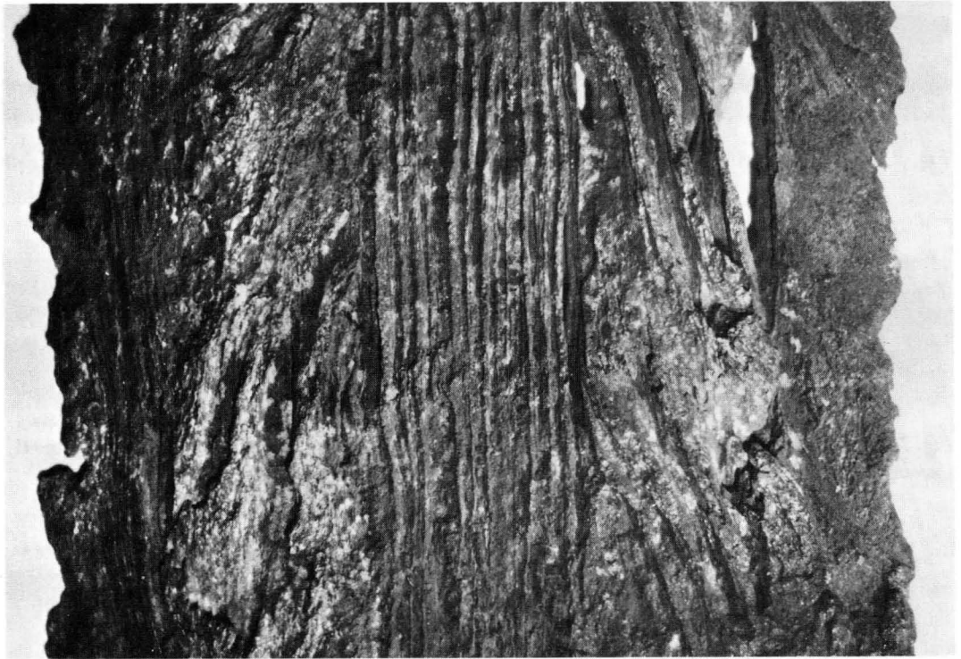
Fig. 7.4a Registration number 1929 2-6 1. L946 Tenth-century Viking sword from the Thames at Windsor. This shows a straight part of the central loop with twists on either side and twisted cutting edges.
