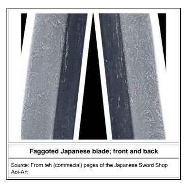
Japanese polishing makes the layered structure well visible. Of course, we can only see it because the welds are stucturally different from the rest.
