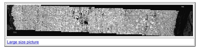
We have a fairly homogeneous piece of ferrite with little carbon but the usual elongated slag inclusions. If the big black "spider" in the middle is a real feature or some artifact of etching is not clear at present. There is no obvious evidence of welding but a closer look does suggest a piled or layered structure produced by fire welding. This is oullined in the .large size picture
