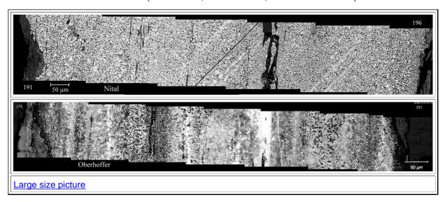
Strong structural changes accross the blade are seen in the Nital etch; they are at least partially due to a changing carbon concentration.
