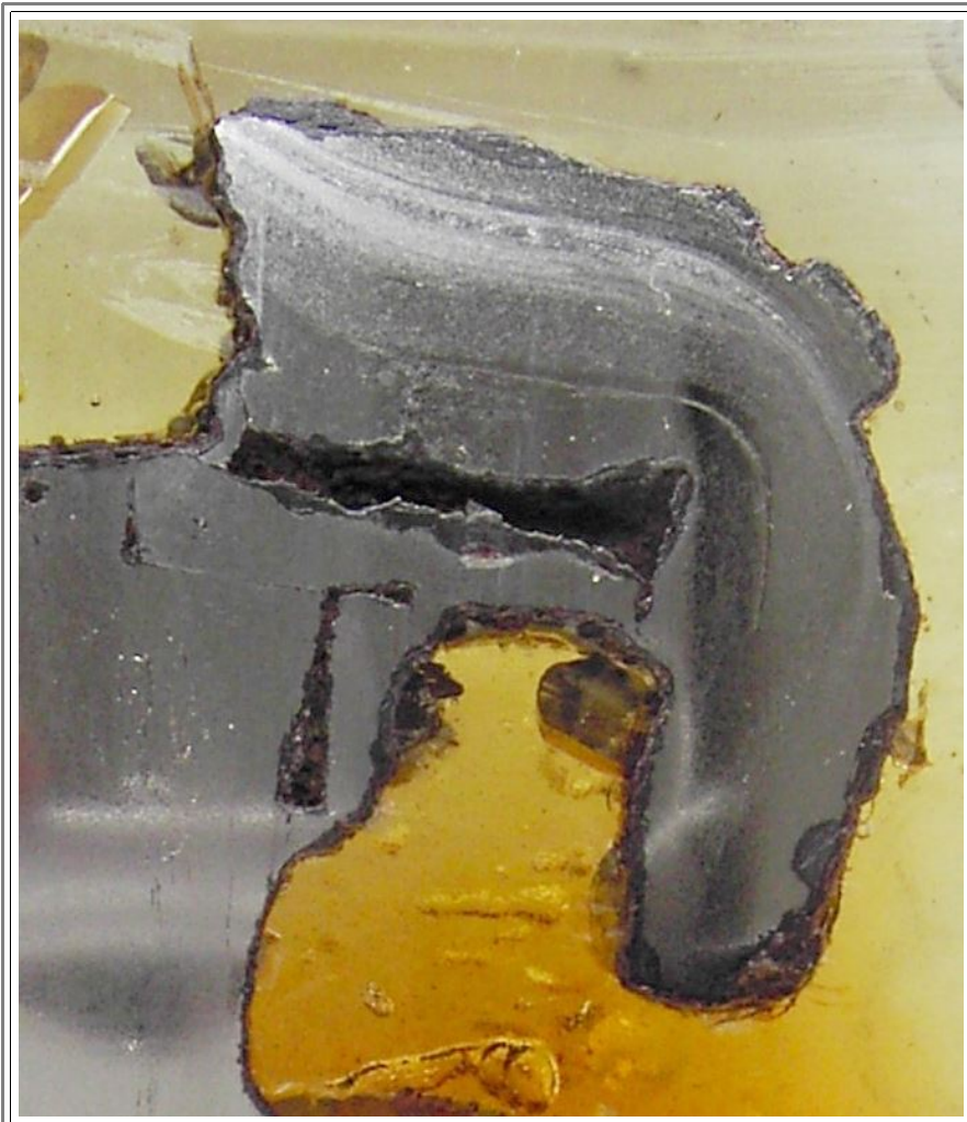
Part of Kiel half; polished and Nital etched. Strongly contrast enhanced.
