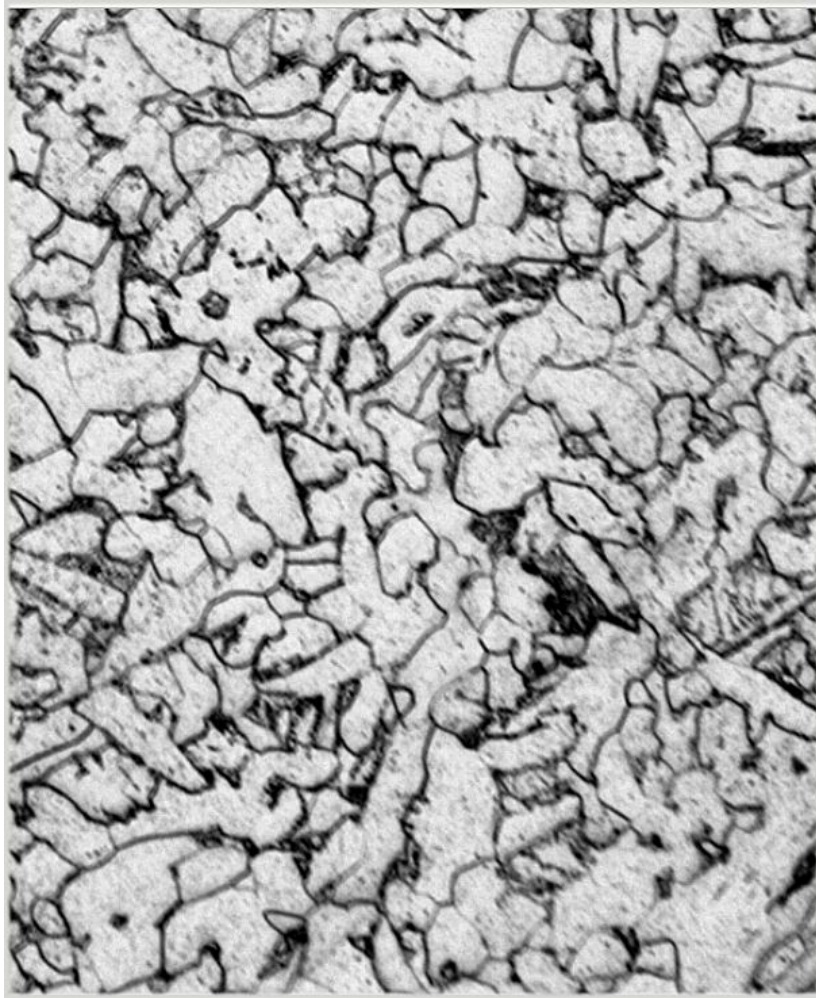
Ferrite structure in region 2
