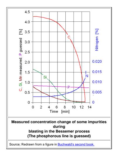
Shown is the measured development of the concentration of carbon (C), silicon (Si) and manganese (Mn) in a 25 ton converter during a 12 minute blast. What phosphorous does is not recorded, the line given is my best guess. Note also the increase of the nitrogen concentration, not to mention the oxygen concentration that is not shown.
