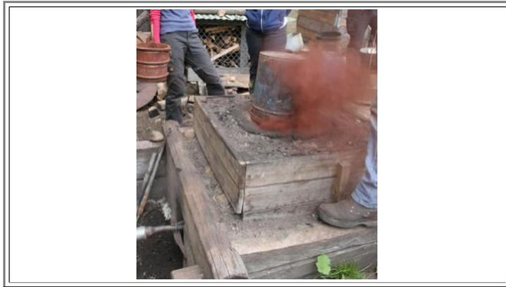
Roasted ore and more charcoal is fed to the top of the furnace at several times.
