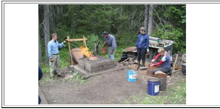
The bloomery furnace is filled with charcoal and it is now running. (It has been preheated over the night). Roasted ore with different properties are mixed together.
