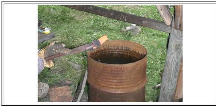
Finally a hardening test. The bar was just on the limit to take hardening - About 0.4% C
