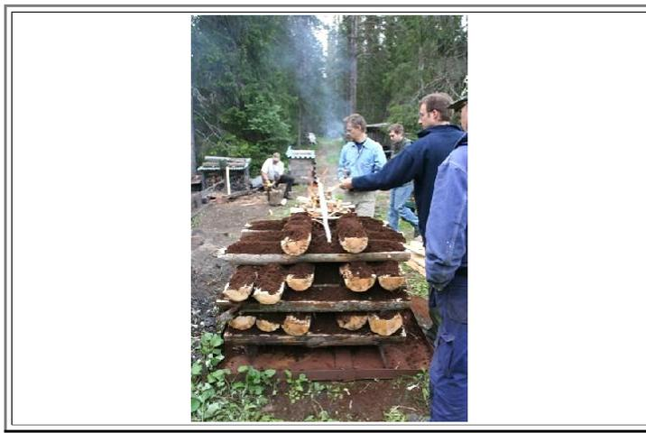
Roasting of the ore is prepared with pine-wood.
