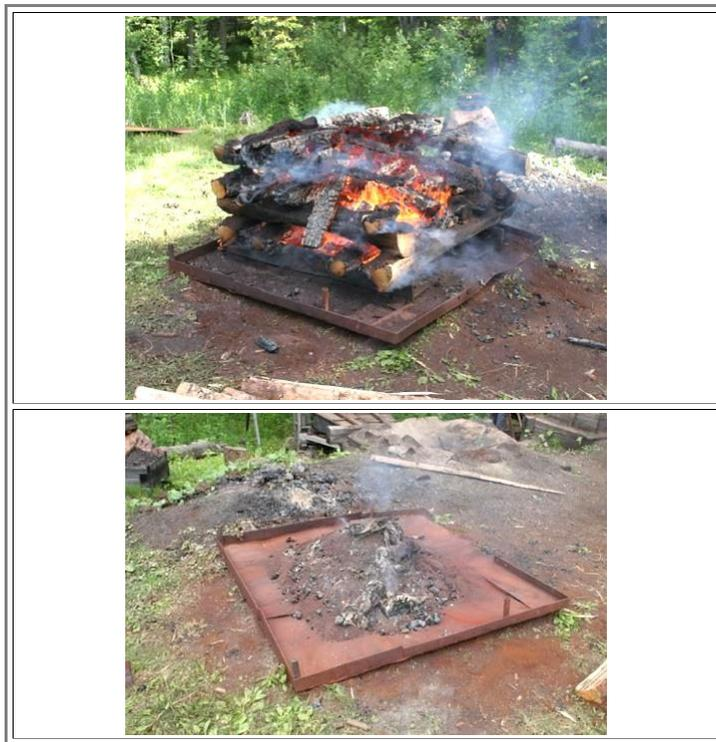
The roasting is completed in three hours. A fine-grain
