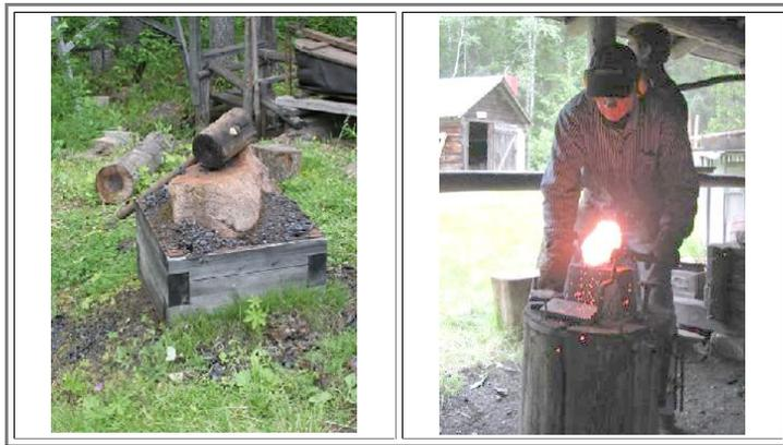
After three and a half hour we got a 3 kg piece of iron and slag (the bloom). It was then consolidated (compacted) by hammering to squeeze out the slag in order to form a solid iron-piece. This work is initially done with a wooden mallet and a stone and then finally with ordinary tools at the smithy.
