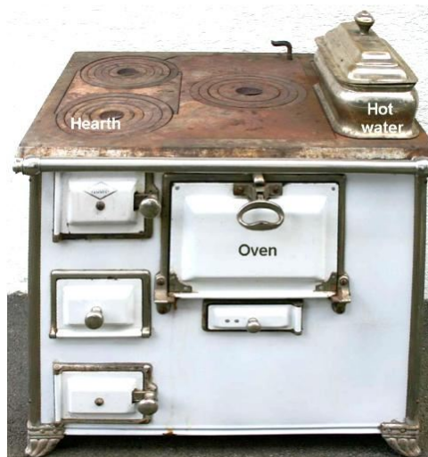
Wood / coal fired kitchen cooking range Remove the rings on top of the hearth and you have an open fire.
