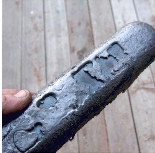
Wrought iron imperfectly coated with cast iron as obtained by "dunking"
