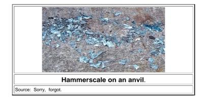
Hammerscale is essentially Magnetite (Fe<sub>3</sub>O<sub>4</sub>). Quite a bit is produced during forging and that limits the time you can heat and bang a piece of iron. It gets smaller all the time.
