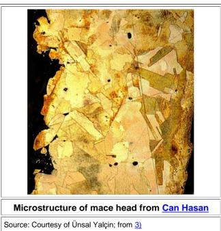
Looking at the microstructure as shown above makes clear (to anybody familiar with <u>typical microstructures of</u> <u>copper</u>) that the object did not solidify (no dendrites), i.e. was not cast. It has been deformed ("pressure twins") and annealed (large grains, straight grain boundaries, few defects in the grains).
