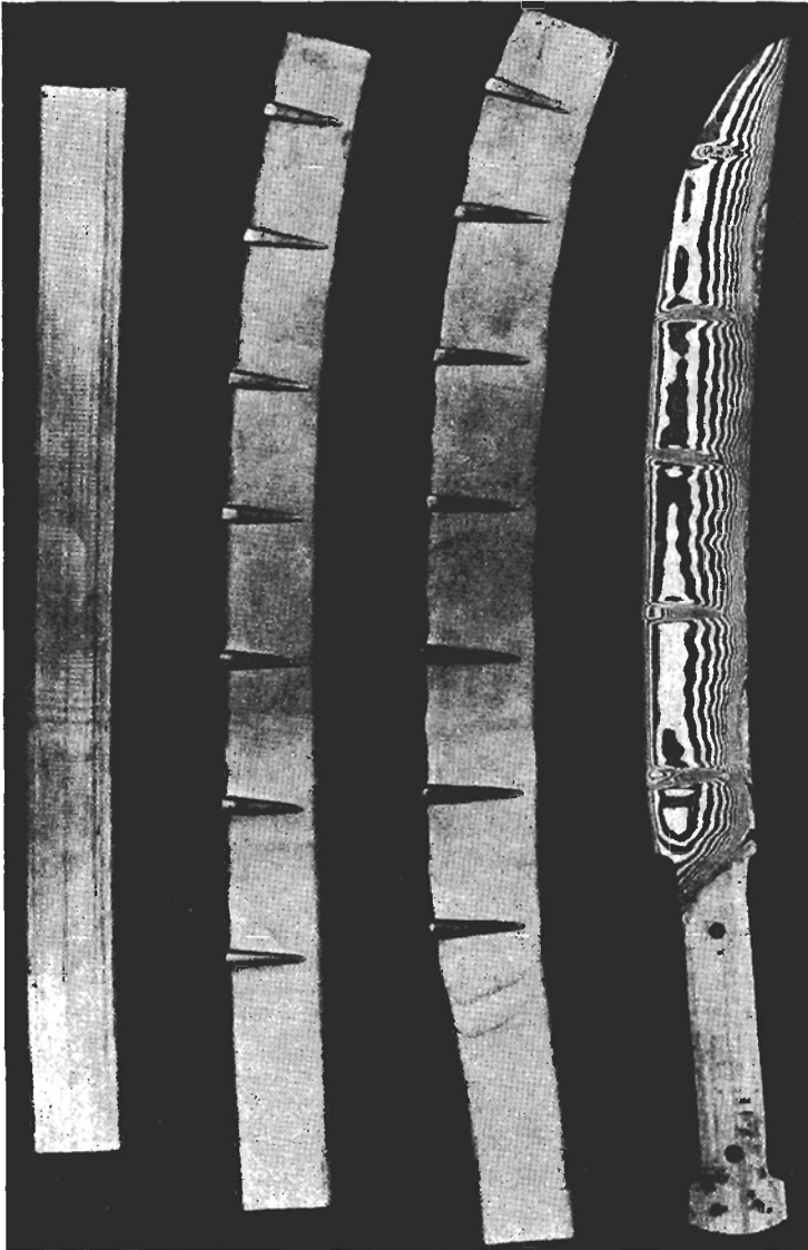
FIG. 46. Manufacturing technique and design produced by means of a swage or chisel having a well rounded edge, worked at an angle to the plane of the bar. In this case, the resulting structure shows a clear analogy to the structure of the original «Kirk Narduban» damascus blade, a magnified detail of which may be seen in Figure 42.
