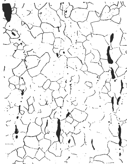
FIG. 49. Pistol barrel of welded damascus, probably of Turkish fabrication.
