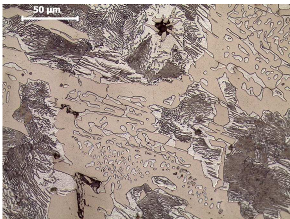
Figure 6. Rhizon steel ingot: microsection at X in Fig. 4, at higher magnification, showing pearlite and ledeburite with slag inclusions. Reproduced by kind permission of M. Biborski and J. Stepiński. Map: iron working sites during the Roman period (after Pleiner, 2000, fig.12).
