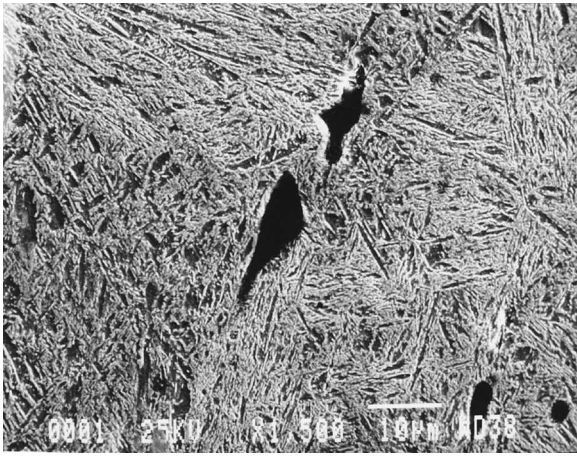
Figure 1. Steel masonry tool tip from Mont Claudianus, 1st to 3rd centuries AD: martensite with glassy slag inclusion.
