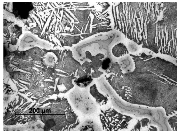
Fig.25 Micro-photograph of sample No.1.2. Ferrite with primal segregation of elements.
