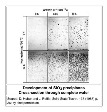
The initial oxygen concentration was 8.15 · 10<sup>17</sup> cm<sup>-3</sup>. The precipitates were rendered visible by <u>defect etching</u>. Shown are just a few out of many pictures for various parameters. Note the denuded zone obtained by a first outdiffusion treatment at 1100 °C (2012 °F) for 10 hours.
