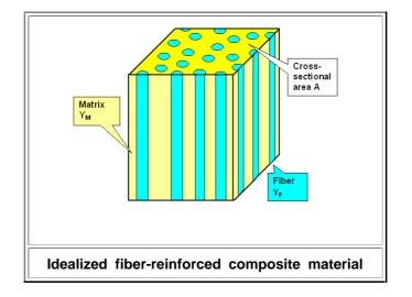
Young's modulus of the fibers we call  $Y_F$ . The matrix goes with  $Y_M$ , and we have  $Y_F > Y_M$ . The total cross-sectional area of the fibers in a cut perpendicular to the fiber direction is  $A_F$ , relative to the total area A.
