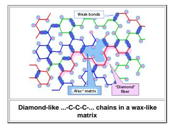
Bingo! As far as Young's modulus is concerned, any polymer is now a composite of diamond-like fibers and a wax-like matrix. The difference between different polymers is due to different volumes of the in-between (large molecules bonded to the carbon atoms take up more room than the small hydrogen atoms in the most simple case of polyethylene), and the arrangement of the fibers (random distribution like a tangle of spaghetti or ordered and parallel).
