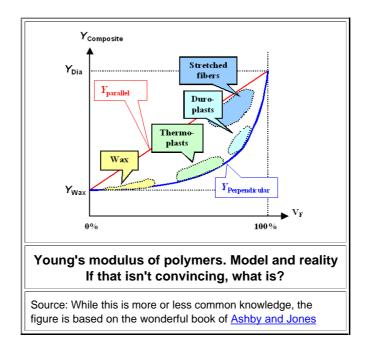
**Thermoplasts** are the (softish) polymers that get soft and more or less liquid when heated a little. Your plastic shopping bag, CD's, plastic containers, etc. are made from thermoplasts. Duroplasts will not get soft upon heating but begin to smolder and stink. Epoxy is an example. Stretched fibers is what you use to tie your ship to the quai.
