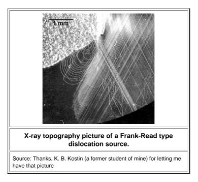
The picture resulted from an of investigation into "<u>wafer bonding</u>", where two Si wafers are placed on top of each other and "bonded", so that a single piece of Si results - with a grain boundary in between. The mottled area in the upper left hand corner shows such a bonded structure, whereas the dark area containing the dislocations as white lines, remained unbonded.
