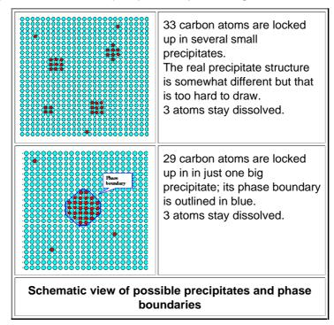
Now a word of warning is in order (<u>once more</u>). Looking at the figure above or others like these, you should realize that there is no such thing as a fully correct drawing of precipitates in crystals.
