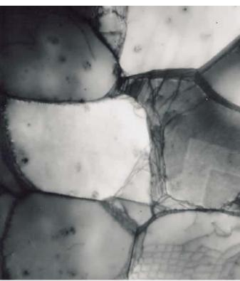
MW -Plate 404 This relatively low magnification micrograph shows the subgrain structure of beaten aluminium foil. Subgrain boundary walls are visible. These are made up of dislocation arrays. The subgrains are about 1µm in size. Inside the subgrains there are many extinction contours. These arise from dynamical electron diffraction effects due to buckling and thickness variations in the
