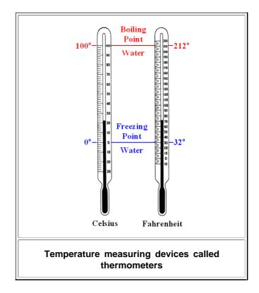
Both thermometers measure the same *thing* ("temperature") but with different *scales*: degree Celsius or degree Fahrenheit.
