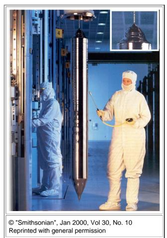
Note that this huge crystal is hanging on a rather thin **Si** seed crystal (see inset). This seed crystal does not only have to support the weight of the crystal, but also the torque needed to rotate the crystal during its growth.
