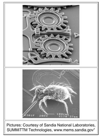
While gear wheels look very good, the real use of **MEMS** so far is in sensors, in particular for acceleration. The sensor exploding your air bag when you wrap your car around a tree is the paradigmatic **MEMS** product.
