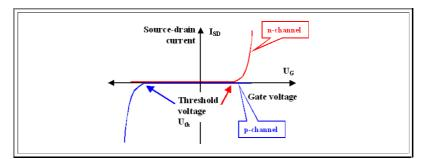
The red curve may stand for a **NMOS** or **n**-channel transistor, the blue one then would be the symmetrical **PMOS** or **p**-channel transistors. The threshold voltages are not fully symmetric if the same gate electrode is used because it depends on the difference of the Fermi energies of the gate electrode materials and the doped **Si**, which is different in the two cases.
