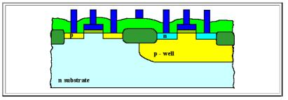
By now, even the "simple" **MOS** technology starts to look complicated. But it will get even more complicated as soon as you try to put a metallization on top. The gate structure already produced some "roughness", and this roughness will increase as you pile other layers on top.
