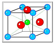
Often, the lattice is not exactly cubic, but slightly distorted. In the case of **BaTiO<sub>3</sub>** this is indeed the case: The **Ti** - ion does not sit in the exact center of the slightly distorted cube, but slightly off to one side. It thus has two symmetrical positions as schematically (and much exaggeratedly) shown below
