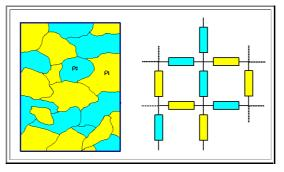
But no matter what kind of volume fraction you use and how you treat the resistor network - the resulting resistivity will *never* be smaller than that of the ingredient with the smallest resistivity.
