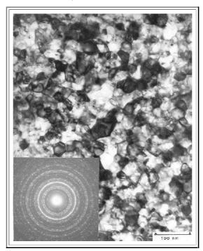
Increasing the annealing time or the annealing temperature makes the PtSi film more coarse grained; this is easily seen in the sequence below. But only the diffraction image shows that an epitaxial relationship to the Si substrate develops at high temperatures.
